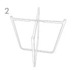
Align the holes at the top and bottom of frame
