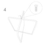
Insert the short screw into the top hole and tighten with hexagonal key provided
